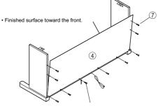
• Fasten the cable holder (9) together with the back panel.
